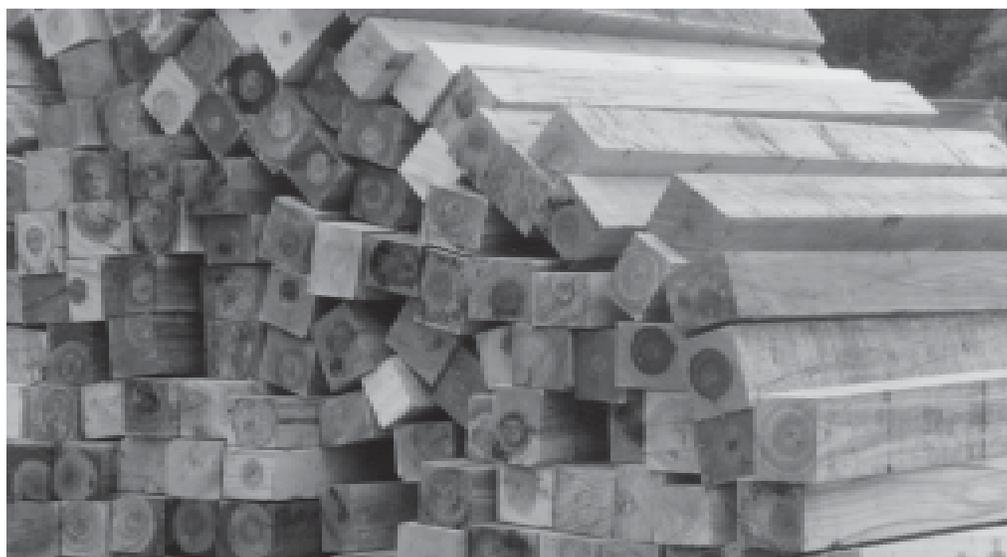
Wood is a cellulose material which can be adversely affected by decay fungi, insects, and marine borers. For all non-durable wood species and the sapwood of all woods, the use of chemical preservatives must be applied to protect wood from attack from these organisms.
