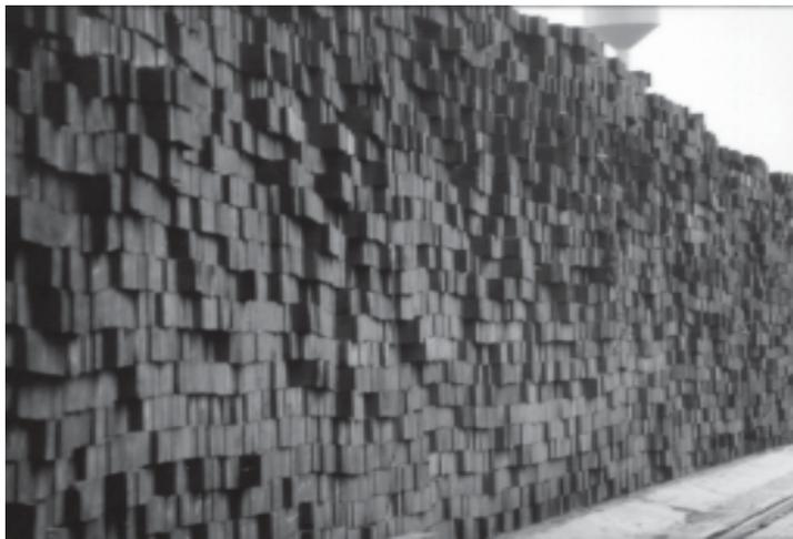
been treated with a creosote solution meeting the requirements of AWP Standard P2. There are also occasions when ties and other timber products such as bridge materials will be treated using the AWP Standard P1/P13 .
